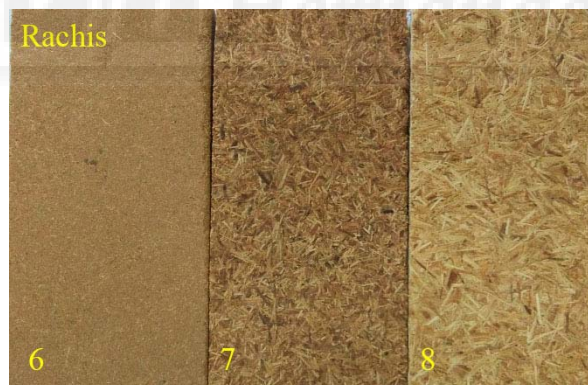
Fig. 9. Particleboards made from rachis of P. canariensis type 7 (<0.25), 8 (0.25-1), and 9 (1-2).
