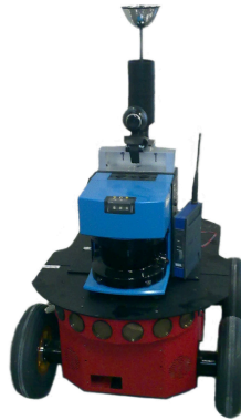
Figure 2.14: Robot Pioneer P3-AT used in this work for the acquisition of omnidirectional images, raw laser data and odometry data.
