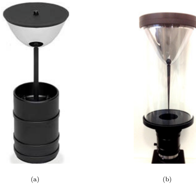
Figure 2.5: Hyperbolic mirrors used in this work, assembled in their coupling systems. Figure 2.5(a) presents the Wide 70 manufactured by Eizho . Figure 2.5(b) presents the Super-Wide manufactured by Accowle .
