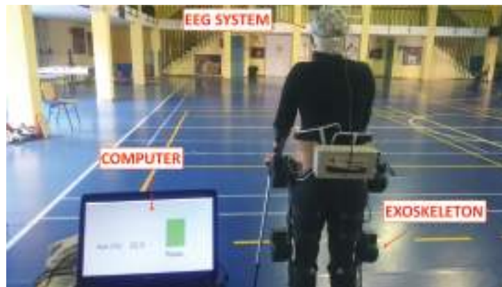
Figure 3. E2 experimental setup. Subjects stood wearing an exoskeleton while their EEG signals were recorded. Once the experiment started, subjects had to relax, clearing their mind as much as possible. Then, a beep auditory signal indicated to the subject to start gait imagery until they heard a double beep auditory signal. After this second beep, subjects had to relax again until the experimental trial finished. Written informed consent was given by the subject to publish the photo.
