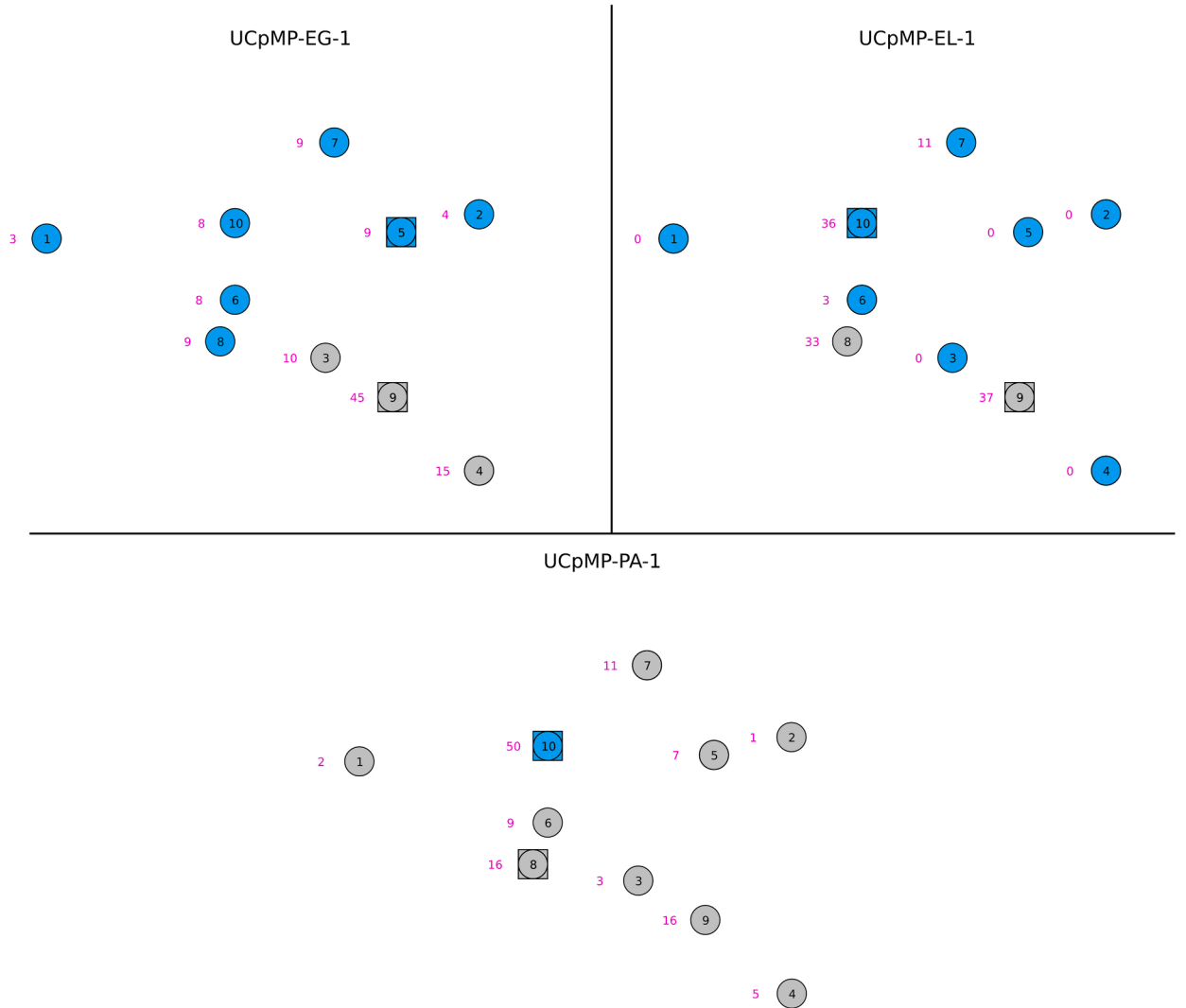
Fig. 4. Solutions of Example 1 obtained with the UCpMP model under different allocation rules with \alpha = \alpha^+ . The three panels correspond to Equal Gain (UCpMP-EG-1), Equal Loss (UCpMP-EL-1), and Proportional Allocation (UCpMP-PA-1). Squares indicate facility locations, colors identify the facility serving each client, and purple numbers denote the allocated demand z_i . (For interpretation of the references to colour in this figure legend, the reader is referred to the web version of this article.)
