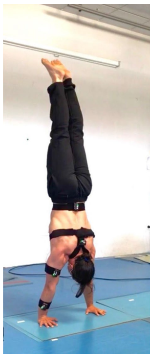
Fig. 1 Shows the set where the measurements were performed, showing the four IMUs and the force platform
