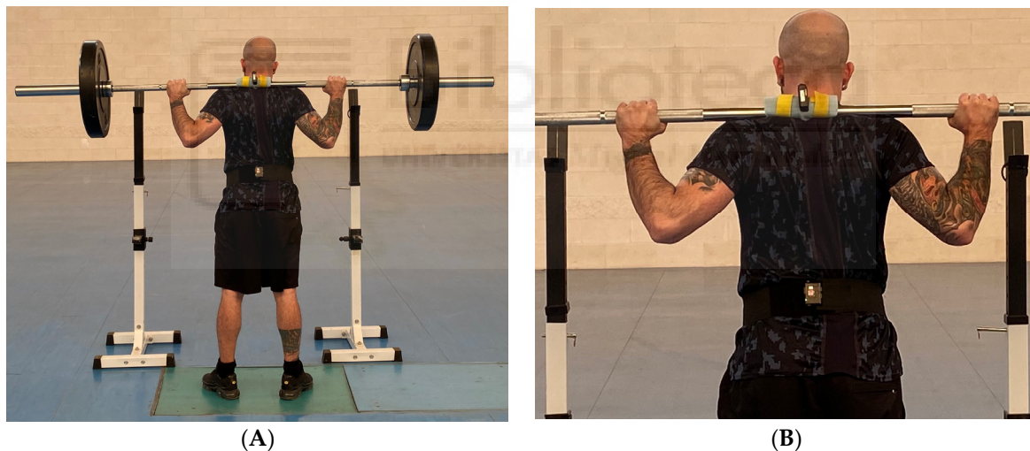
Figure 2. Equipment setup: (A) overview; (B) placement of the IMUs: one located at the bar and one at L5.
