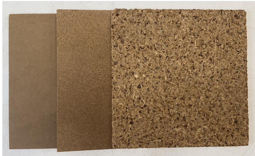
Figure 2. Particleboards manufactured with 3 particle sizes (from left to right: type A, type B, and type C).
