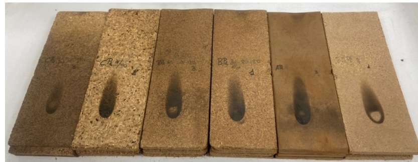
Figure 6. Some specimens of Canary Island palm trunks used in the reaction-to-fire test.
