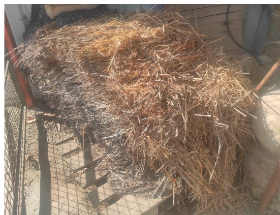
Figure 1. Sorghum waste used for manufacturing the experimental boards.
