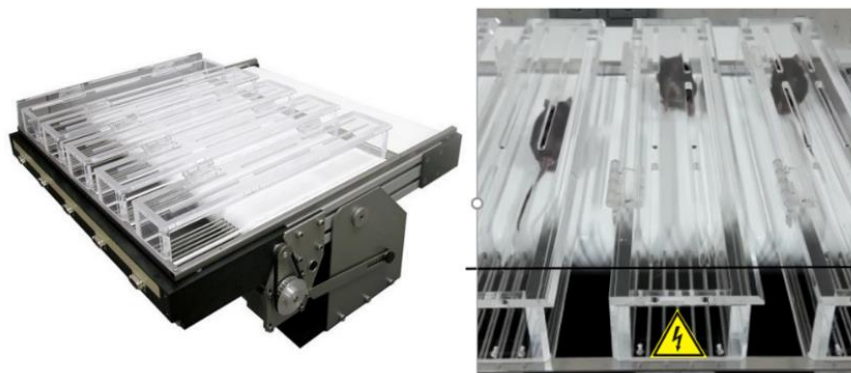
Figure 17. Treadmill apparatus for mouse running. Five-line treadmill device was used to train the mice daily for 3 weeks. Mice run at a speed of 9-12 m/min and received a mild shock (0.4 mA) when arriving at the end of the belt to motivate to keep running.
