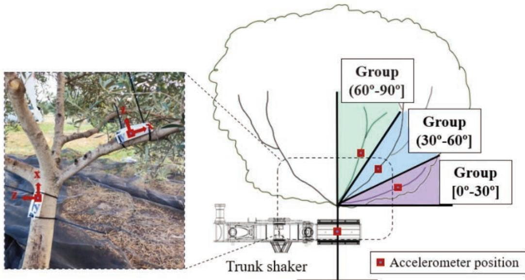
Figure 2. Real position (left) and schematic (right) of the acceleration sensors on the tree.
