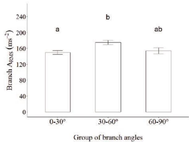
**Figure 4.** Acceleration RMS measured in tree branches according to the group of branch angles (mean and standard error). Differences between letters indicate significant differences (ANOVA,  $p < 0.05$ ; *post-hoc* Student’s *t*-test with Holm correction,  $p < 0.05$ ).
