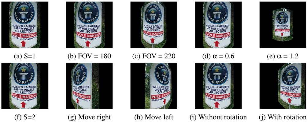
Figure 2: Synthetic fisheye images with data augmentation.
