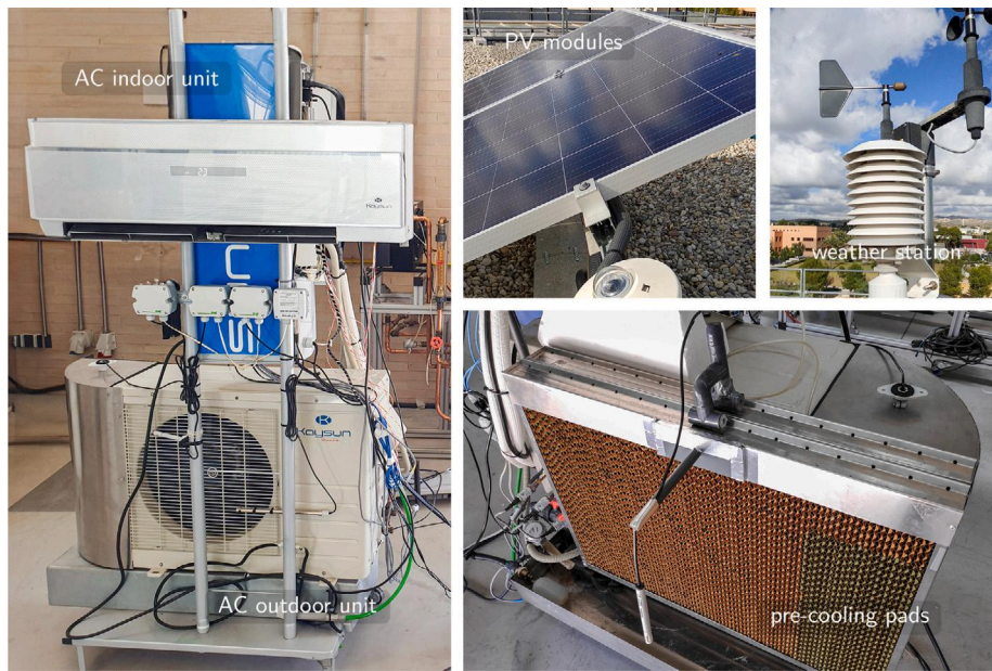
Fig. 1. Prototype of a solar cooling system with evaporative pre-cooling pads.
