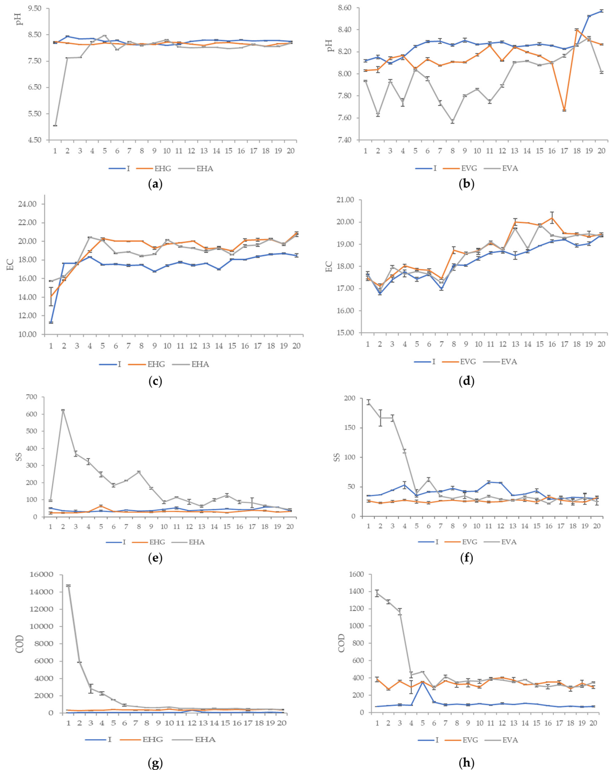
Figure 3. pH, EC, SS and COD results of horizontal and vertical water flow bioreactors. (a) Weekly pH (units) of horizontal water flow bioreactors. (b) Weekly pH (units) of vertical water flow bioreactors. (c) Weekly EC ( \text{mS cm}^{-1} ) of horizontal water flow bioreactors. (d) Weekly EC ( \text{mS cm}^{-1} ) of vertical water flow bioreactors. (e) Weekly SS concentration ( \text{mg L}^{-1} ) of horizontal water flow bioreactors. (f) Weekly SS concentration ( \text{mg L}^{-1} ) of vertical water flow bioreactors. (g) Weekly COD concentration ( \text{mg L}^{-1} ) of horizontal water flow bioreactors. (h) Weekly COD concentration ( \text{mg L}^{-1} ) of vertical water flow bioreactors.
