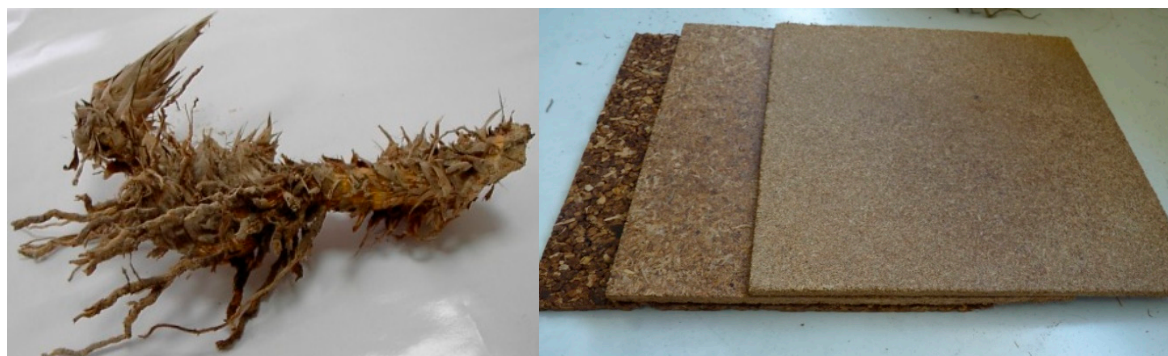
Figure 1. Arundo donax L. rhizome and binderless rhizome particleboards.
