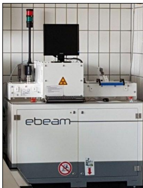
Figure 16. e-Beam instrument used for pre-treatment of plastics
