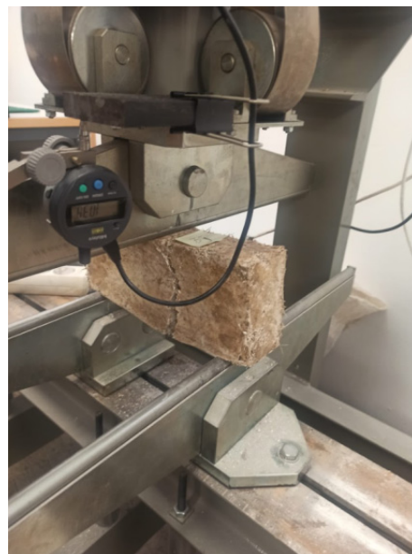
Figure 6. Universal Testing Machine—flexural test.
