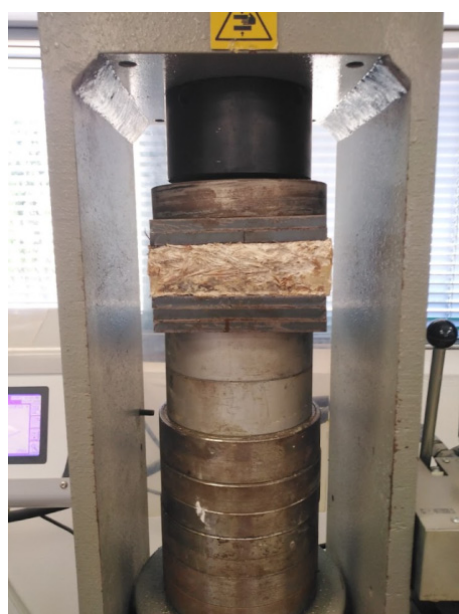
Figure 7. Universal Testing Machine—compressive strength test in type E specimens.
