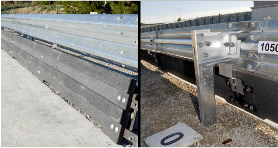
Figure 5. Front and rear view of the original prototype of MPS.
