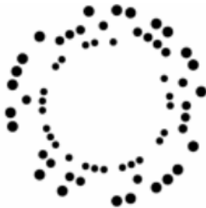
Figure 2.8 Example of RuneTag marker, RUNE-129. Extracted from [12].
