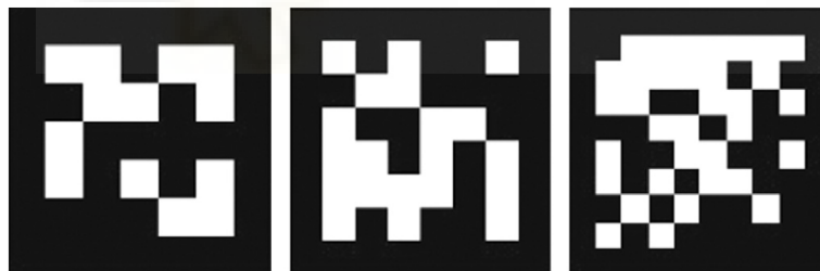
Figure 2.5 Example of ArUco markers generated with different grid sizes. Extracted from [8].
