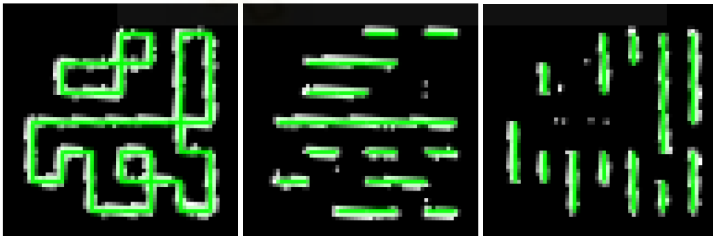
Figure 5.4 Examples of border detection of 6X6 ArUco marker in cases with all edges, only horizontals, and only verticals.
