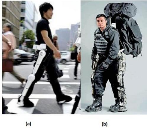
*Figura 6: a) Hybrid Assistive Limb (HAL), b) Berkeley Lower Extremity Exoskeleton (BLEEX)*
