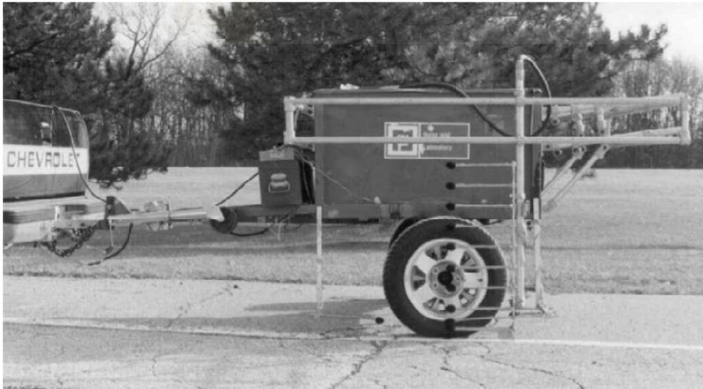
*Figura 10: Near-Field Acoustic Array Technology (NAAT) [16]*
