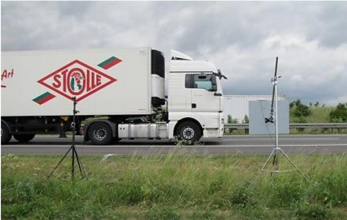
*Figura 8: Método Statistical Pass-By [6].*
