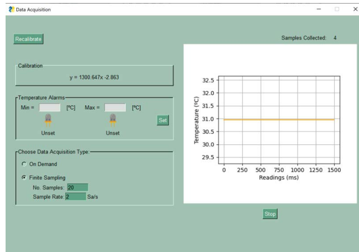
Fig. 3.7.20 Ongoing finite sampling acquisition with the parameters: 20 samples and 2 Sa/s
