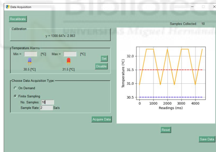
Fig. 3.7.21 finite sampling acquisition finished with the parameters: 10 samples and 2 Sa/s
