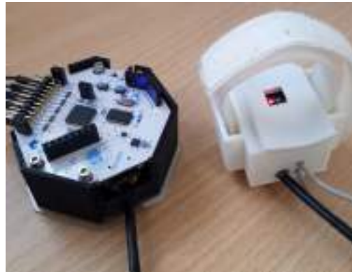
Figure 5. Black case in which the OpenBCI board is attached with screws and just below the board there are the power supply for the system (9 V battery) and the Atmega328p microcontroller. On the lower part of the case there are two Velcro strips so that it can be placed on a strap around the user's waist.
