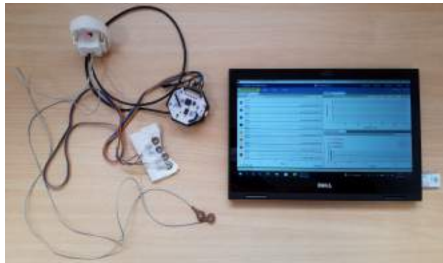
Figure 6. Ambulatory monitoring system with the tablet.
