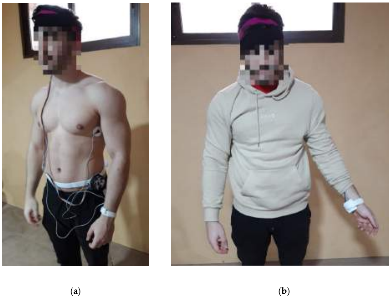
Figure 7. (a) Placement of each of the elements that make up the ambulatory monitoring system on the user; (b) Final arrangement of the ambulatory monitoring system on the user with clothing. It can be seen that the design is unobtrusive and produces practically no disturbance to the user's daily activities.
