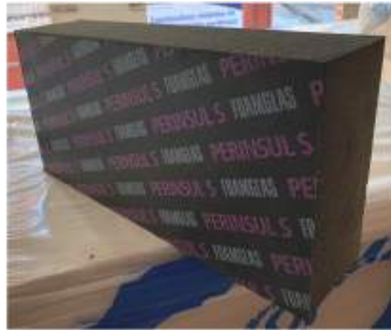
Fig. 7. M3 improvement considered to reduce the thermal bridge of waffle slab fronts. Properties of the materials listed in Table 3 (the rest of the layers coincide with those indicated in Fig. 4). Left: diagram of the M3 improvement. Right: detail of the cellular glass block.
