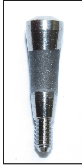
FIGURE 1: Image of the healing abutment used in this study, which received the surface treatment in the transmucosal portion.
