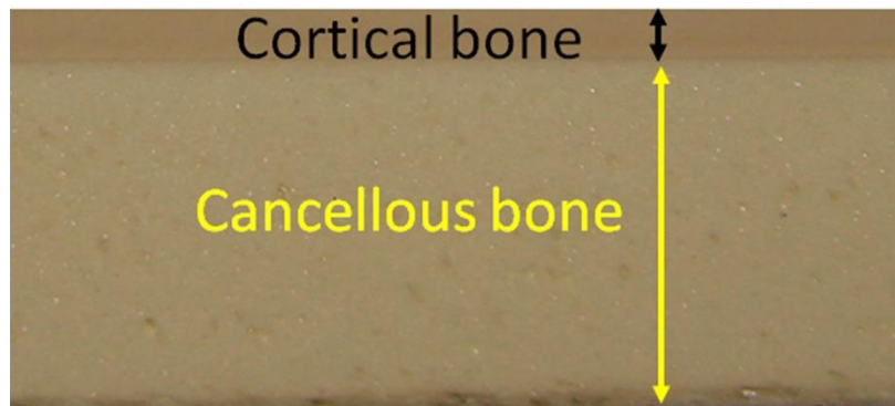
Figure 1. Representative image of the synthetic bone blocks showing the cortical portion (black arrow line) and cancellous bone portion (yellow arrow line).
