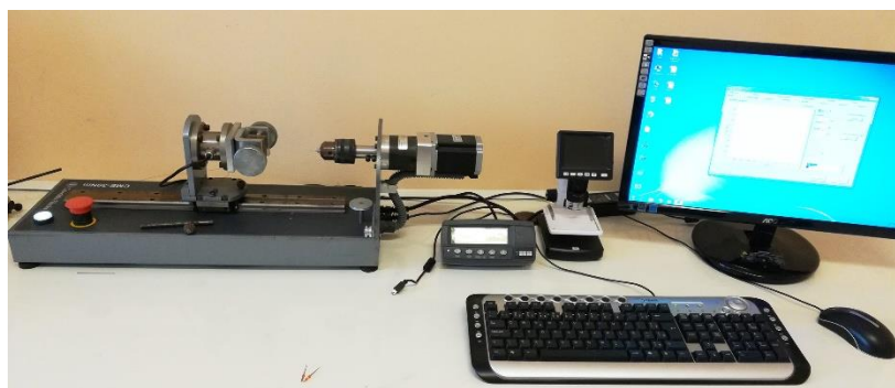
Figure 5. Image of the torque machine used to install and remove the implants into the synthetic bone blocks.
