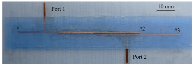
Fig. 5. Photograph of the fabricated filter before its implementation is completed. On top of the structure resonator #2 can be clearly seen.
