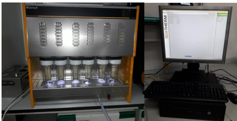
Figura 20. Extractor Soxhlet J.O, Selecta Mo.6003286.
