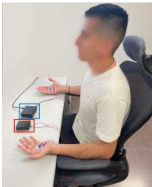
Figure 6. Experimental setup during EDA signal acquisition. The subject is simultaneously connected to the AC excitation device, indicated in blue, and the DC excitation system, marked in red.
