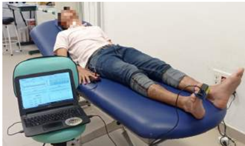
Figure 9. Subject in supine position and configuration of the measurement acquisition system and a computer with the data display interface.
