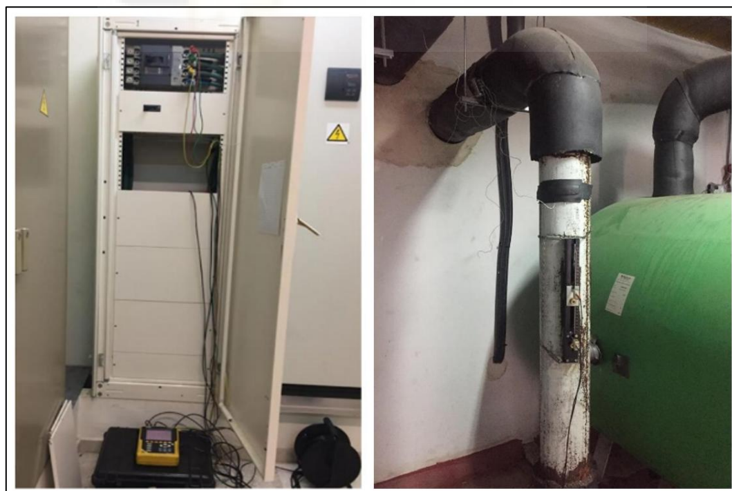
Figure 27. Meters used in the study. Power meter (left) and flow meter with thermocouples (right)
