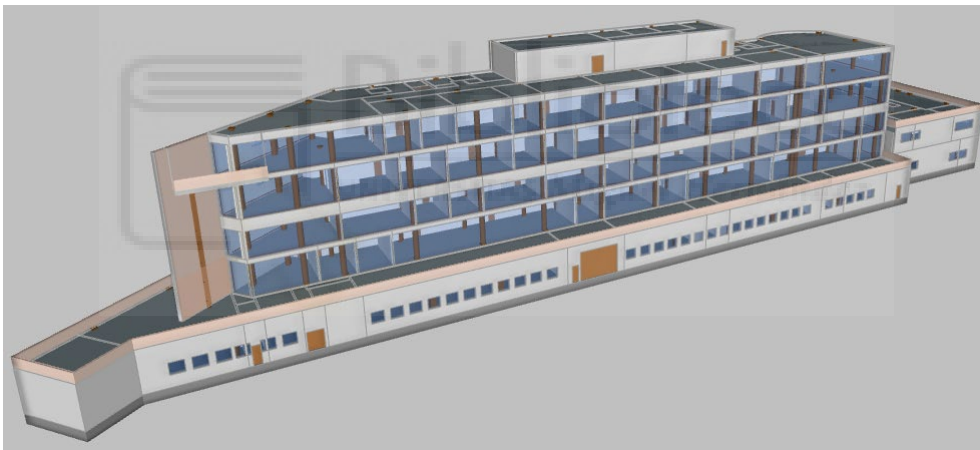
Figure 2. Building energy model – View of the rear façade.
