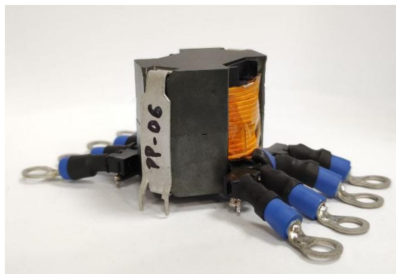
Figure 39. Fully assembled RM14-3C95 push-pull transformer with (d) distribution.
