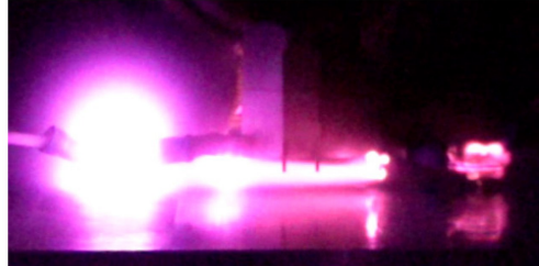
Figure 11. DCX transformer: Corona discharge at 1 mbar.
