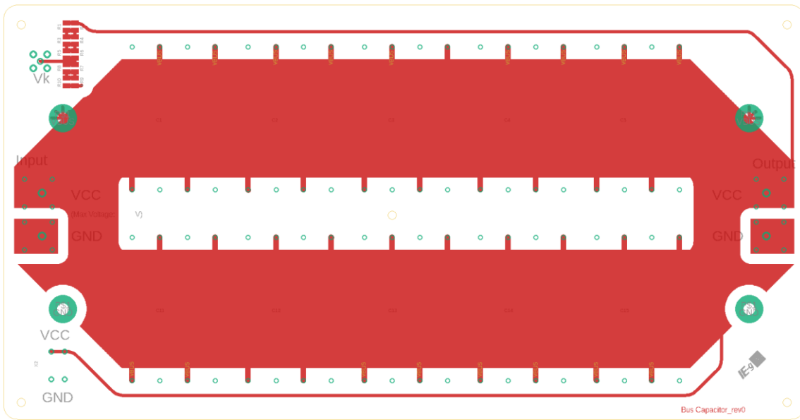
Figure 93. Bus capacitor board – Top layer.
