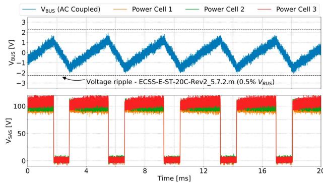
Figure 8. Experimental 3s1p S3DCX. Top: distribution bus voltage (AC mode). Bottom: Solar Array Section voltage.
