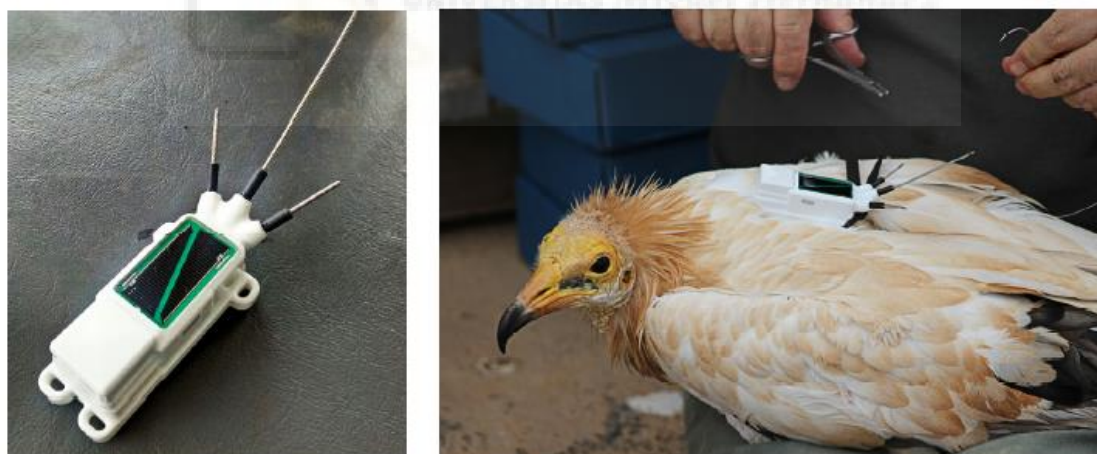
Figure 6: Details of an e-obs device on the left and a Canary Egyptian vulture being equipped with an e-obs device on the right. Photography © J. A. Donázar (left) and M. García-Alfonso (right).
