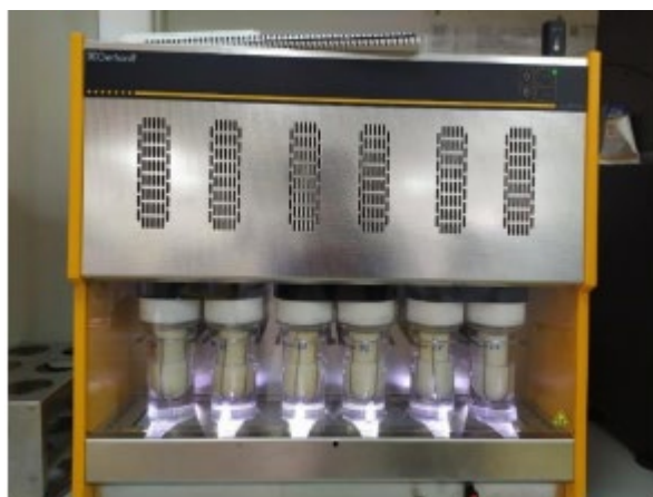
Figura 4. Extractor Soxhlet J.O, Selecta Mo.6003286
