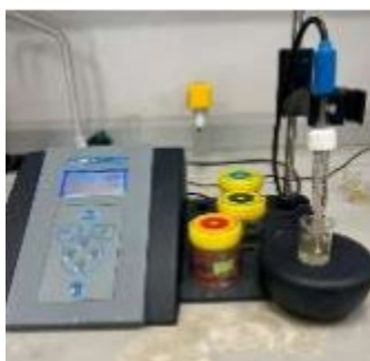
Figura 6. pH-metro GLP 21 Crison (Eutech Instruments Pte Ltd., Singapur)
