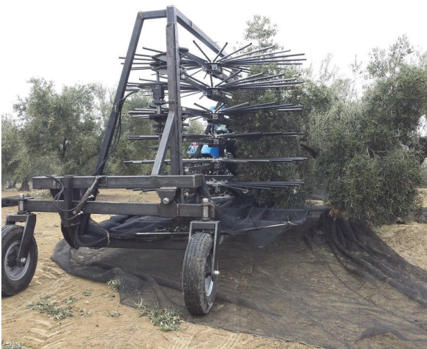
Figure 1. Prototype of lateral canopy shaker harvesting a traditional olive tree.
