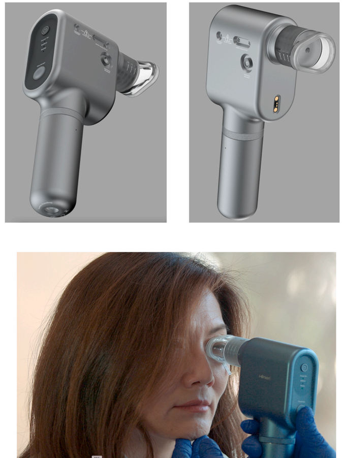
Fig. 1. A. The i-Onion™ instrument. B. Application of the instrument to the orbital margins of a subject's right eye. In this example, the Schirmer test strip has been placed to illustrate how tear flow is measured.
