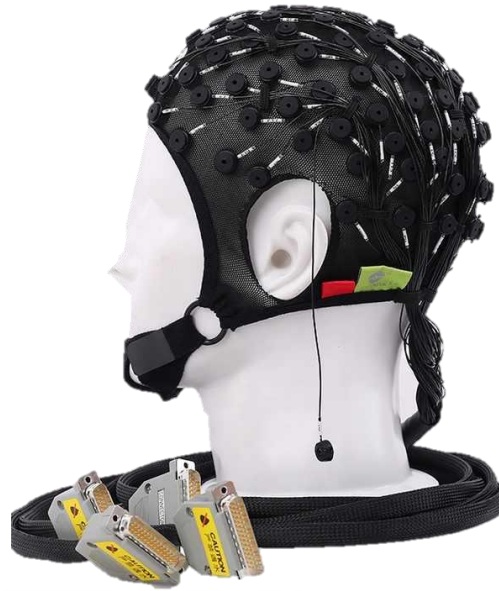
Appendix 1. EEG cap with 126 electrodes.
