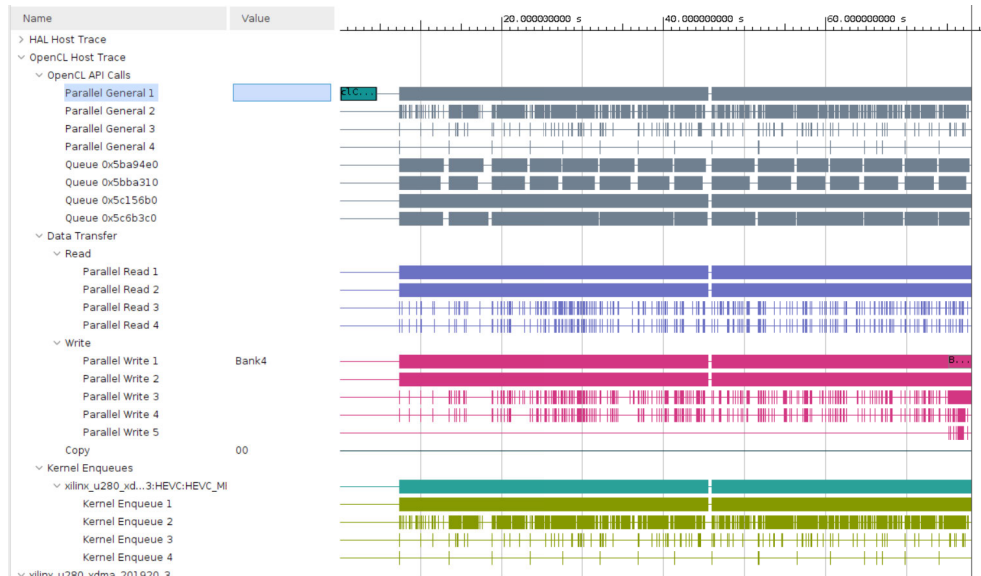
FIGURE 8. Vitis Analyzer profile of the first 16 frames of Cactus video sequence using an IME module with four HW units.
