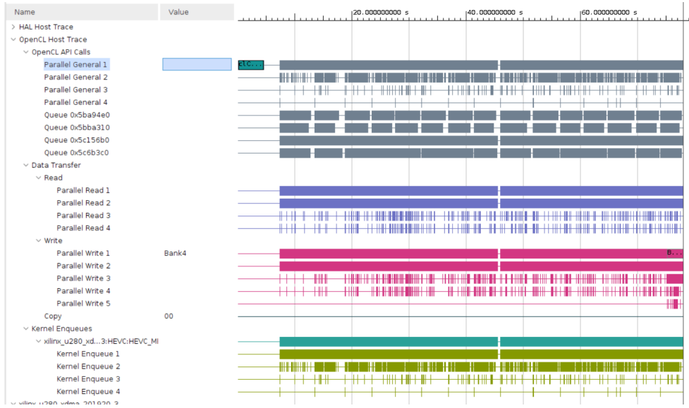
FIGURE 8. Vitis Analyzer profile of the first 16 frames of Cactus video sequence using an IME module with four HW units.
