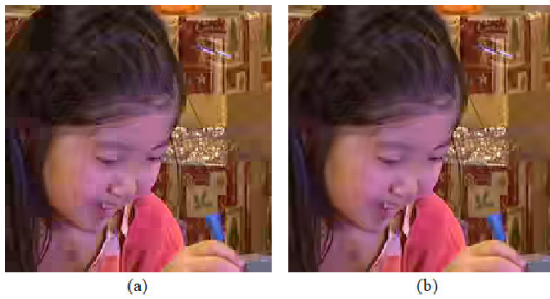
FIGURE 2. Example of using deblocking filter in BlowingBubbles frame, encoded at QP37: (a) DB disabled, (b) DB enabled.
