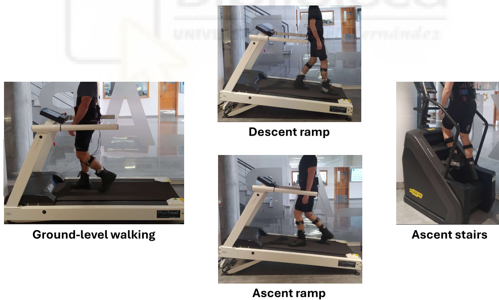
Figure 4.8: The performed gait activities and the experimental setup used to estimate the vGRF are represented in the images.
