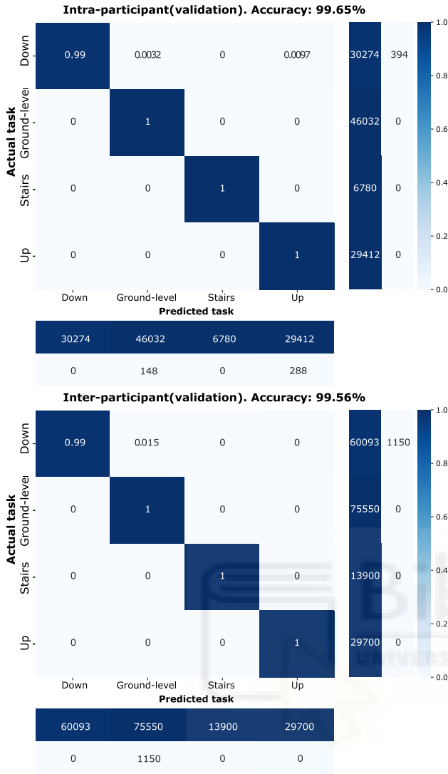
Fig. 4. Confusion matrices obtained with the proposed CNN classifier for intra-participants and inter-participants. The rows of the matrix show the ADL that was performed, and the columns show the ADL that was predicted. The matrices include the four gait ADLs that were done in the experiment: walking on a flat surface, going up a ramp (Up), going down a ramp (Down), and climbing stairs.
