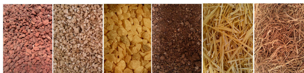
Figure 3. Some inorganic and organic materials that can be part of a technosol: volcanic crushed rock, perlite, gravel limestone rock, sewage sludge compost, hay straw and crushed palm leaf, from left to right (photographs taken by the authors).
