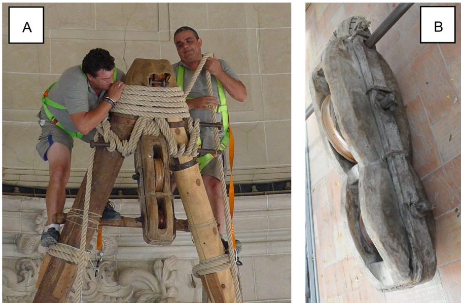
Fig. 7 Pulleys. A Fixing the pulley to the crane. B Double pulley designed to raise and lower 2 different devices
