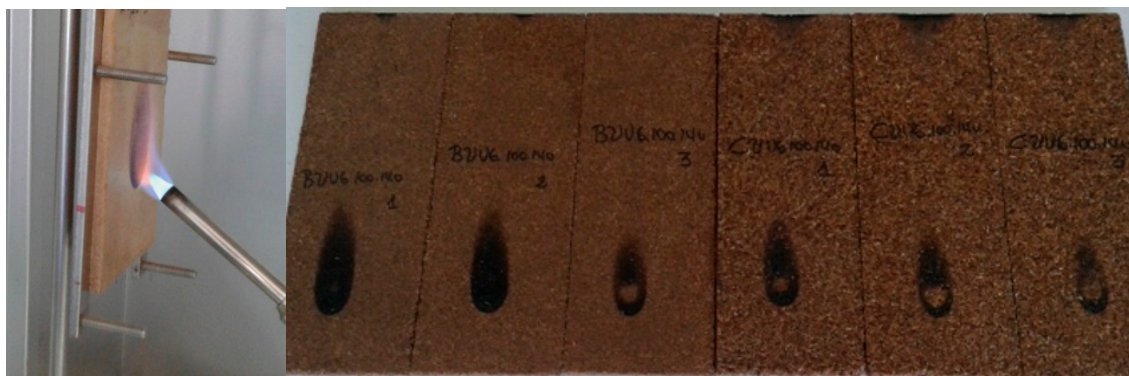
Figure 2. Sample placed on the frame and samples used in the reaction-to-fire test.
