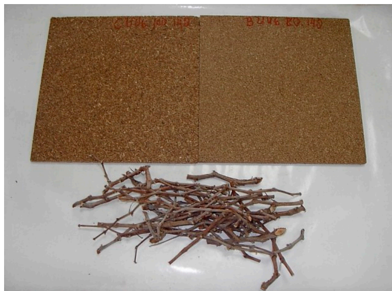
Figure 1. Vine prunings and samples of the manufactured boards (300 × 300 mm 2 ).
