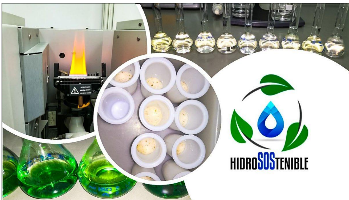
Figure 13. Digestion and minerals determination through atomic absorption and emission spectrometer
