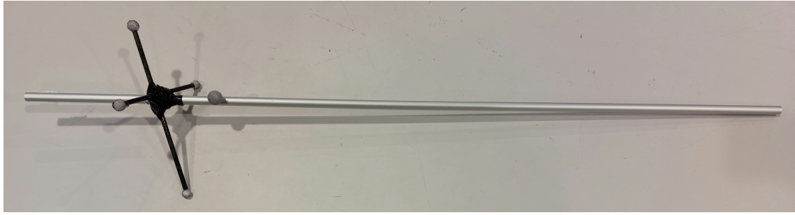
Figure 6.1 Stick with markers for the motion capture system to simulate the relative movement between the LiDARs and a power-line.
