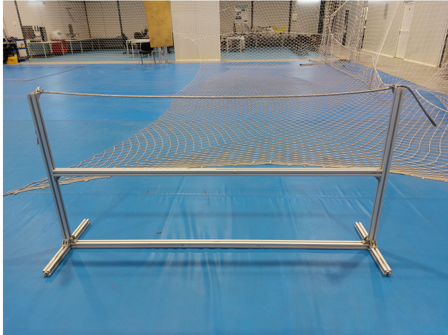
Figure 6.9 Mock power-line used for the flight experiments.
