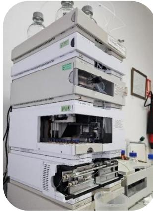
**Figura 15.** HPLC (Agilent HPLC 1200 Infinity).
