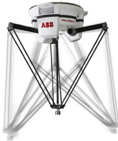
Figura 5. Robot delta ABB IRB 360
