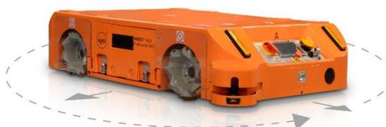
Figura 7. Robot móvil MOBOT AGV FlatRunner MW (004)
