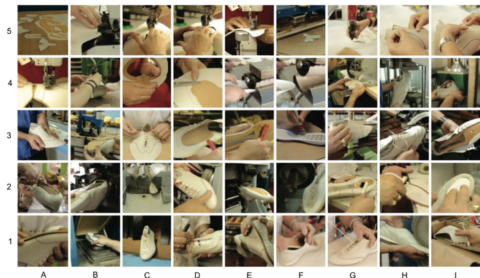
Figure 1. Steps to produce a pair of shoes. Courtesy of Simplicity Works Europe.
