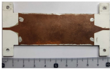
Fig. 10. Top view of the fabricated DSRW with l_2 = 7.0 cm for TE 10 mode excitation.
