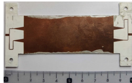
Fig. 14. Top view of the fabricated DSRW with l_2 = 7.0 cm for TE 20 mode excitation.
