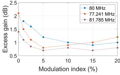
**Fig. 3.** Excess gain for the observed ML threshold, in dB, at different shifting frequencies  $f_s$  and electrical modulation indices  $\mu$ . Zero modulation index refers to a situation where the AOFS is driven by a single RF tone without AM, for which ML induction at  $f_s = 80$  MHz was not possible in our laser.
