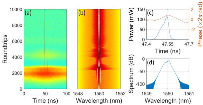
**Fig. 6.** Same as in Fig. 5 but with a loss of 16 dB and triggered by AM ( $\mu = 0.005$ ) during the first 5000 recirculations. The final pulse width is 58 ps (FWHM). See **Visualization 2**.
