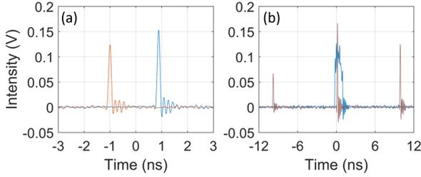
**Fig. 4.** (a) Pulse intensity in self-starting ML emission at the integer resonant condition (orange) and AM-triggered ML at  $f_s = 80$  MHz (blue). (b) Pulse cluster (blue) generated by AM-triggered ML and its drift (brown) when the AM is turned off.
