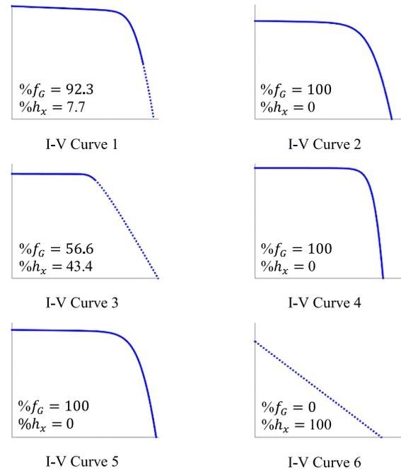
Fig. 8.  $I$ - $V$  curves with the  $I$ -approach and actuation percentage of  $f_G$  and  $h_x$ .
