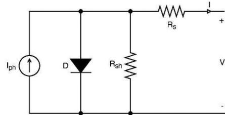
Fig. 1. PV module SDM electrical circuit.
