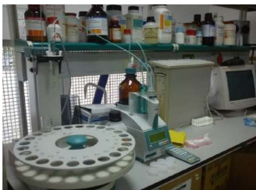
Figura 14. pH-metro Metrohm 760 Sample Changer
