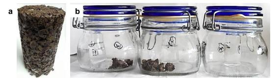
**Figure 9 - a:** Aspect of the mixture after being taken from the reactor; **b:** hermetic jars with sample and CO2 traps.
